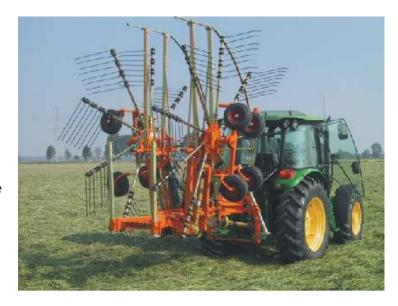
safety devices of the hydraulic hoisting cylinders from the driver's seat and lower the rotors to start working. The correct working position and machine balance are found by adjusting the height of the tractor hoisting device and the third point position in order to let the teeth pass just over the ground.
